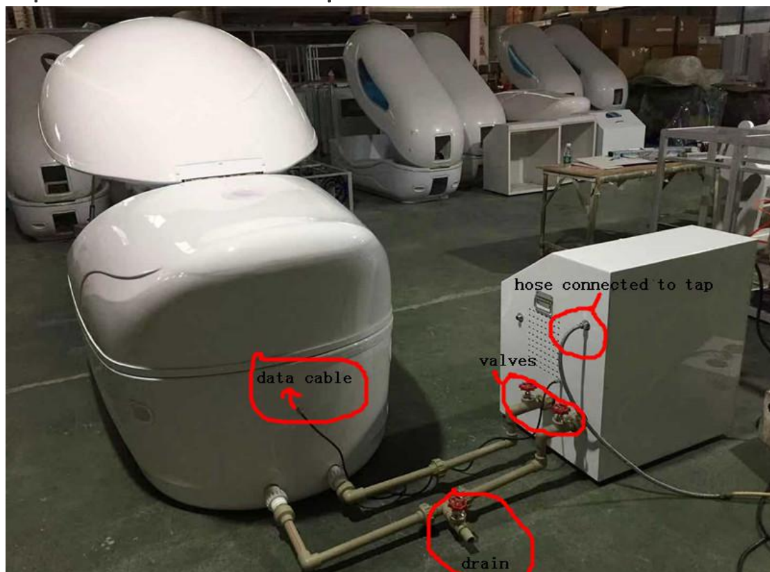
Pipe connection of new pod:
